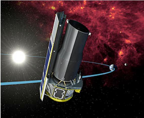
The Spitzer Space Telescope (formerly SIRTF, the Space Infrared Telescope Facility) was launched into space by a Delta rocket from Cape Canaveral, Florida on 25 August 2003. During its mission, Spitzer will obtain images and spectra by detecting the infrared energy, or heat, radiated by objects in space between wavelengths of 3 and 180 microns (1 micron is one-millionth of a meter). Most of this infrared radiation is blocked by the Earth's atmosphere and cannot be observed from the ground.
