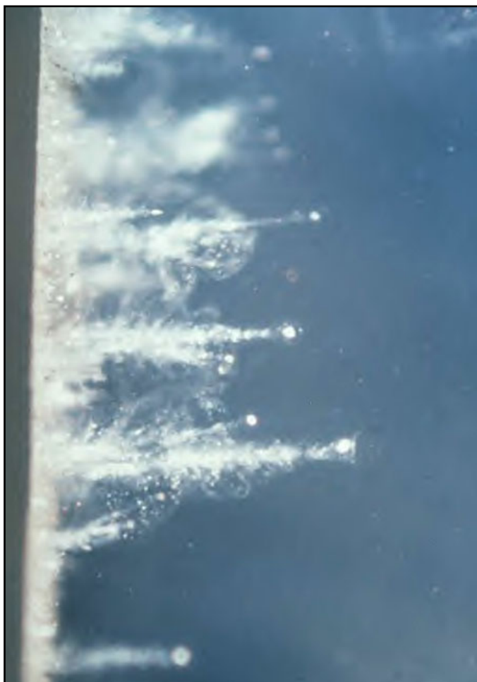
The Stardust spacecraft used a grid holding aerogel to capture dust particles from comet Wild 2. In this test, high velocity dust particles are stopped unharmed at the end of cone shaped tracks in a sample of aerogel
